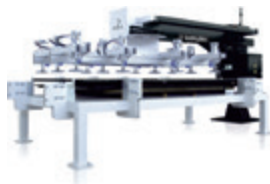
Loading Unit: Automatic loading via rotary swing arm. Individually controlled vacuum cups. Verifies sheet thickness with cutting program.
