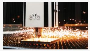
What stops others from delivering ultrahighpower lasers? Short cutting head life due to contamination on optical lenses. The patented eVa® cutting head solves the problem, delivering power and reliability.
