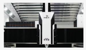
**Carbon Fiber Bridge:** Designed to be short, light, vibration dampening and is driven from the center of mass to maximize machine Gs.
