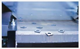
**Integrated conveyor:** Ensures no fallen parts are damaged by subsequent cutting.
