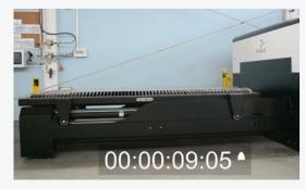
**Pallet exchange in 9 seconds:** It is servo, not hydraulically driven, and repeatable on reinsertion to 0.003 inches.
