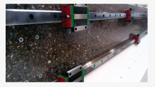
**Polymer Granite Base:** Each of the two sides weigh over 8,000 lbs. They are temperature stable, rigid, and vibration dampening for high G motion.
